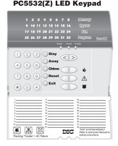
The **PC5508, PC5508Z, PC5516** and **PC5516Z** Keypads are available 1. applications with fewer than 32 zones. The functions explained in this manual are the same for all three LED keypad types.
